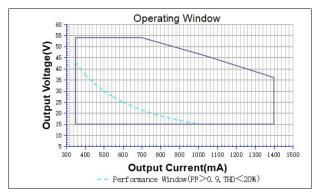
It's important to set the output current (AOC value) according to the LED voltage and make sure the power is within 50 W + 5%.
