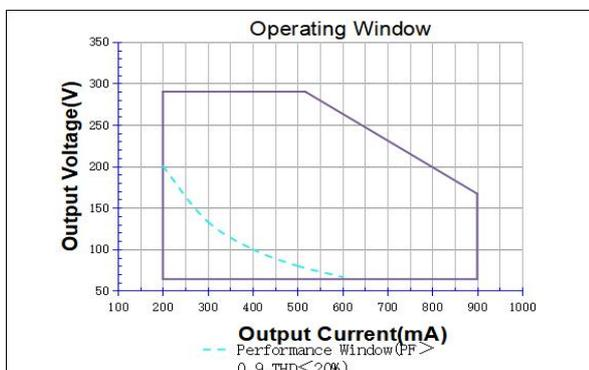
It's important to set the output current (AOC value) according to the LED voltage and make sure the power is within 150 W + 5%.
