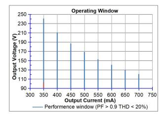
It's important to set the output current (AOC value) according to the LED voltage and make sure the power is within 84 W + 5%.
