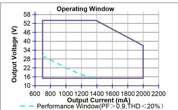
It's important to set output current (AOC value) according to LEDs voltage, make sure the power is within 75W +5%
