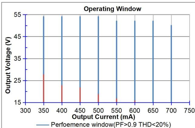
It's important to set output current (AOC value) according to the LED voltage, make sure the power is within 35W +5%
