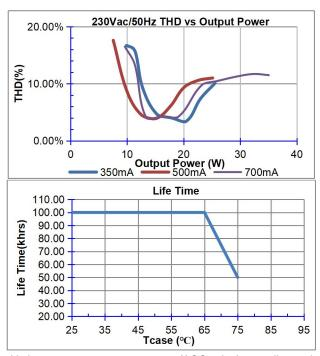
It's important to set output current (AOC value) according to the LED voltage, make sure the power is within 35W +5%
