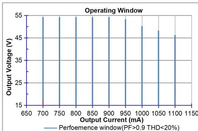
It's important to set output current (AOC value) according to LEDs voltage, make sure the power is within 50 W +5%
