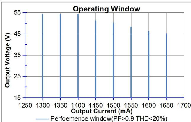
It's important to set output current (AOC value) according to the LED voltage, make sure the power is within 75 W +5%
