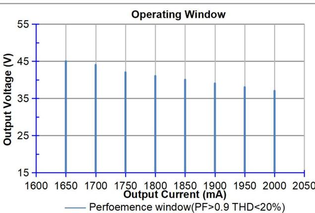
It's important to set output current (AOC value) according to LEDs voltage, make sure the power is within 75 W +5%
