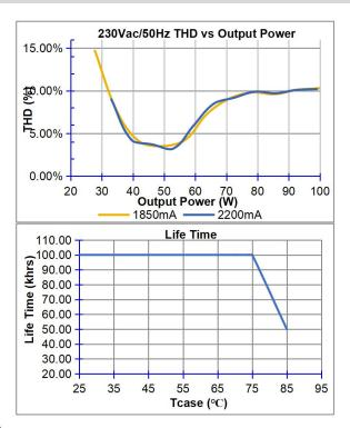
It's important to set output current (AOC value) according to LEDs voltage, make sure the power is within 100W +5%
