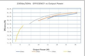
It's important to set the output current (AOC value) according to the LED voltage and make sure the power is within 36 W + 5%
