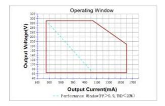
It's important to set the output current (AOC value) according to the LED voltage and make sure the power is within 300 W + 5%.
