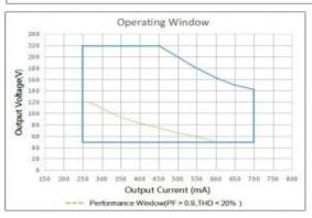
It's important to set the output current (AOC value) according to the LED voltage and make sure the power is within 300 W + 5%.
