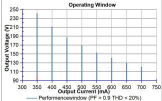
It's important to set the output current (AOC value) according to the LED voltage and make sure the power is within 84 W + 5%.
