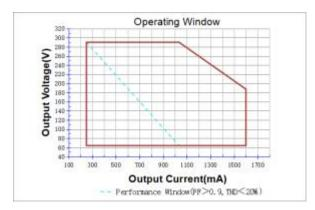
It's important to set the output current (AOC value) according to the LED voltage and make sure the power is within 300 W + 5%.
