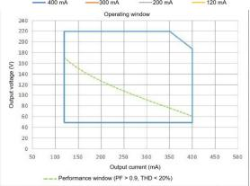
It's important to set the output current (AOC value) according to the LED voltage and make sure the power is within 300 W + 5%.
