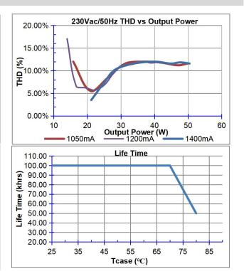
It's important to set output current (AOC value) according to LEDs voltage, make sure the power is within 50 W +5%
