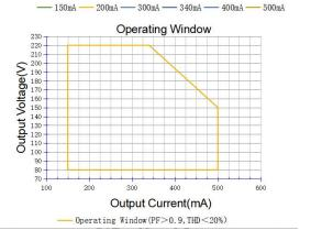
It's important to set the output current (AOC value) according to the LED voltage and make sure the power is within 75 W + 5%.
