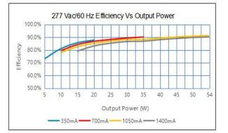
It's important to set the output current (AOC value) according to the LED voltage and make sure the power is within 54 W + 5%.
