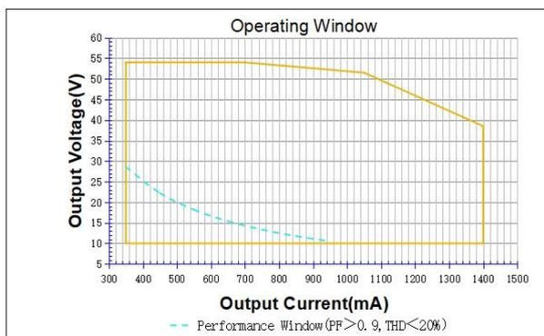
It's important to set the output current (AOC value) according to the LED voltage and make sure the power is within 54 W + 5%.
